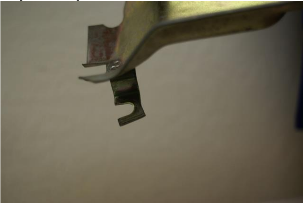
Showing the rear hook that goes on the bolt head:
