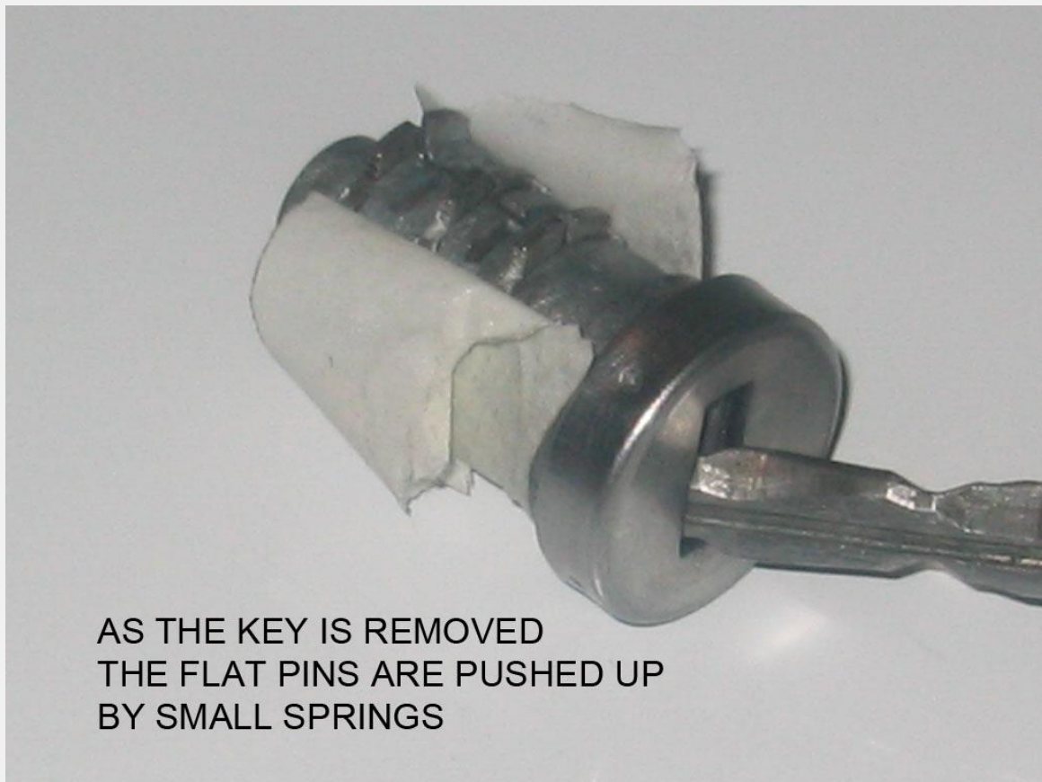
Barrel with alarm core, actuator, and spring
