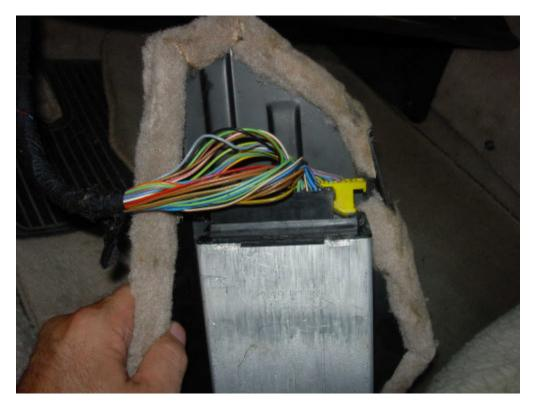
3. Disconnect the wiring harnesses from the controller. These are 25 pin keyed connectors. The connectors are keyed in opposite directions.
