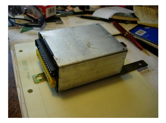
5. To open the enclosure requires using the screwdriver to pry the aluminum tabs  $(4 \log - 4 \text{ short})$  out enough to clear the plastic face panel.
