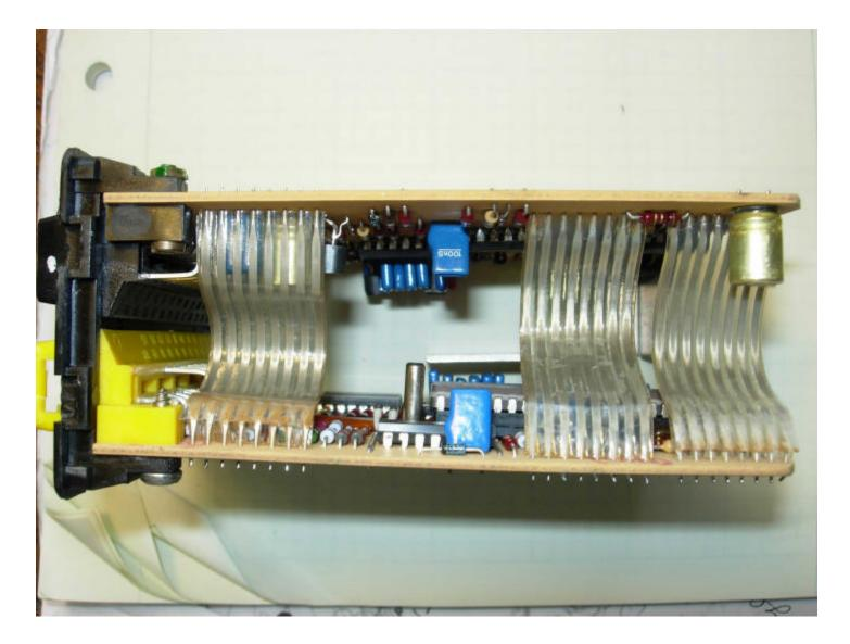
9. Inspect the assembly for broken parts and corrosion. Does the circuit board or components look burned or the surround area is black or dark brown? Does the enclosure and assembly SMELL burnt? This can indicate a component failure or something shorted.
