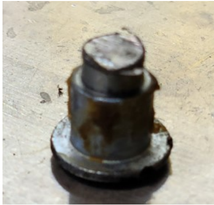
The roller bolt must be ground out of the arm
