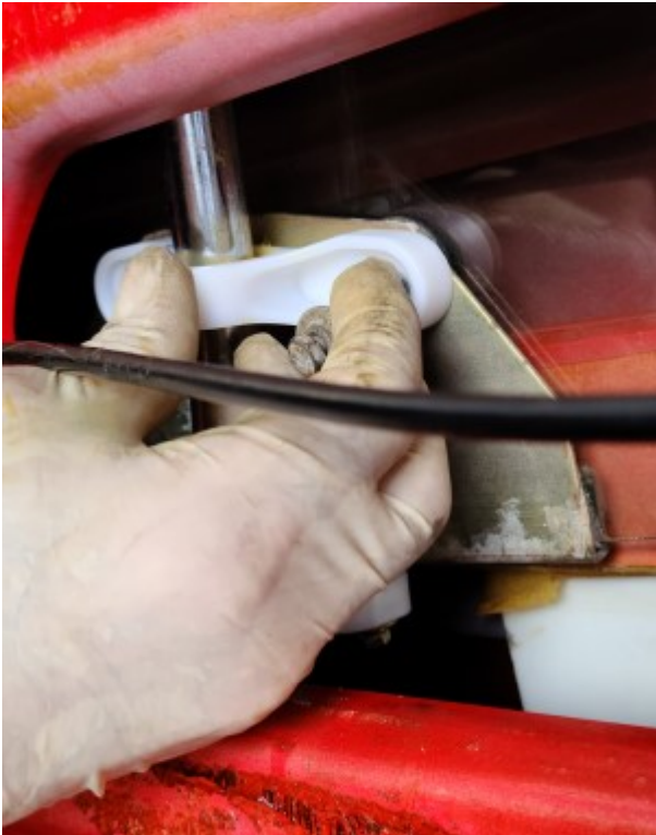
The upper slide is being installed. Here it is visible how the slide bolts to the widow plate.
