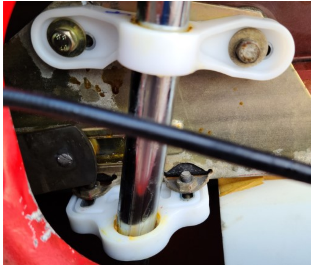
The upper and lower slides are installed.
