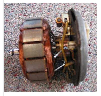
Place assembly into housing, remembering the washer and the small spring tab on the side.
