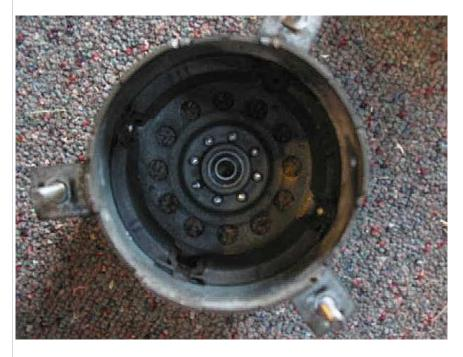
Reassemble rear plate onto motor with brushes retained. Remove nails. If you only just put the nails through the top hole on the brush housings they are very easy to remove
