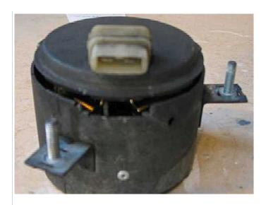
Place holding tabs back in position. I used a cold chisel for this.
