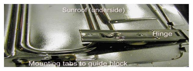
Around the edge of the sunroof is a rubber gasket. The rear gasket is held in place by a plate bolted onto the rear of the sunroof. The plate can catch on the edges bending and preventing smooth operation. Since the gasket is not designed to be a weather proof seal there is no reason to glue it in place. If the frocking is coming off the remainder can be removed with a little lacquer thinner. Before installing the sunroof be sure the rubber gasket is securely in place.
