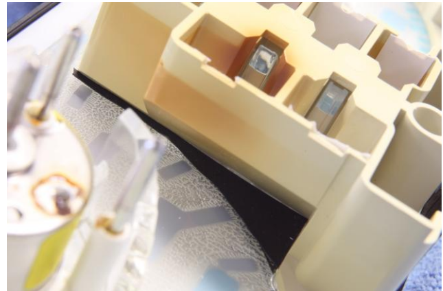
Figure 15: Black tape added to help prevent analog gauge backlighting from bleeding into A/T selector lever position indicators
