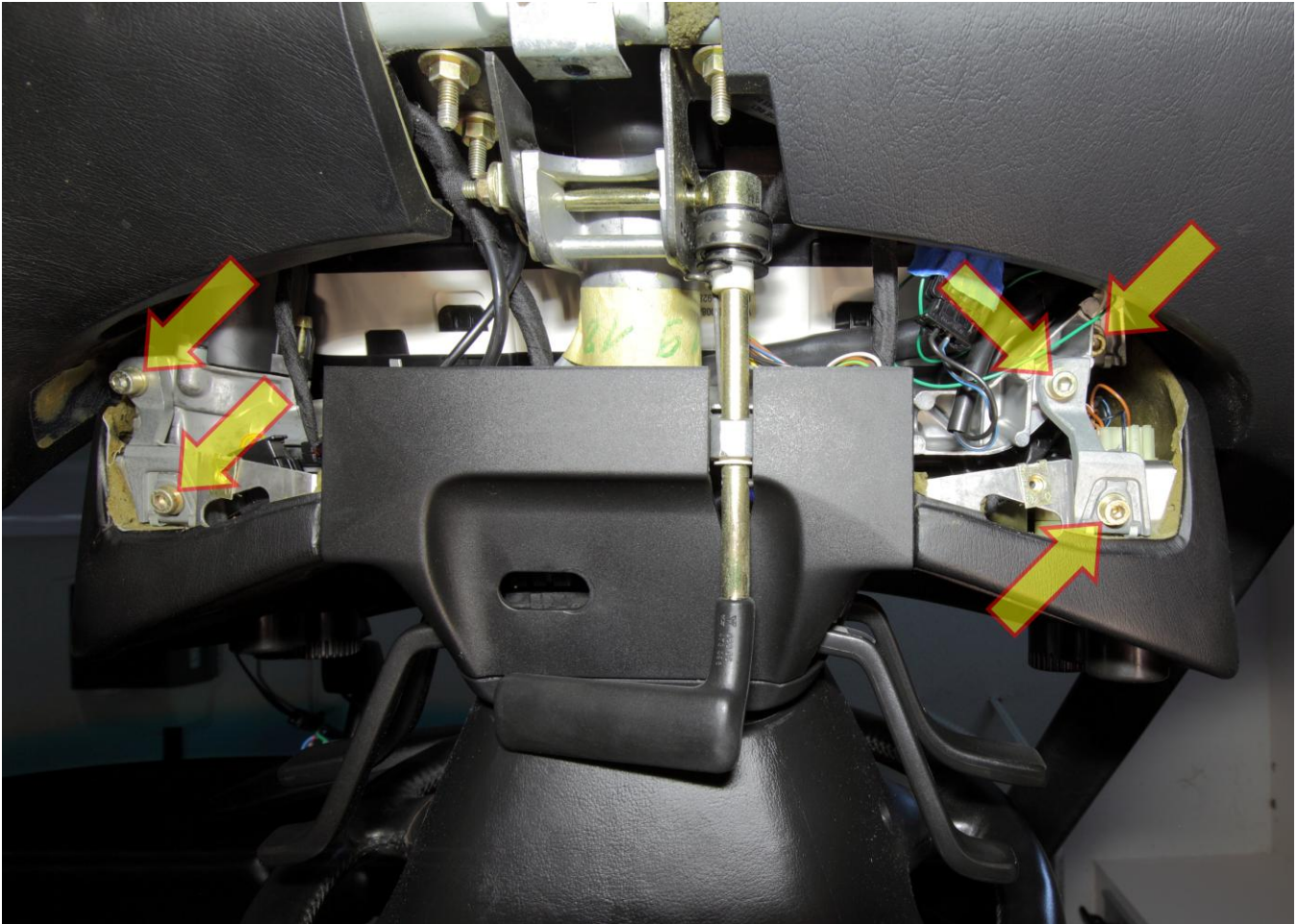
Figure 2: Looking up at the bottom of the instrument pod and the five screws that secure it
