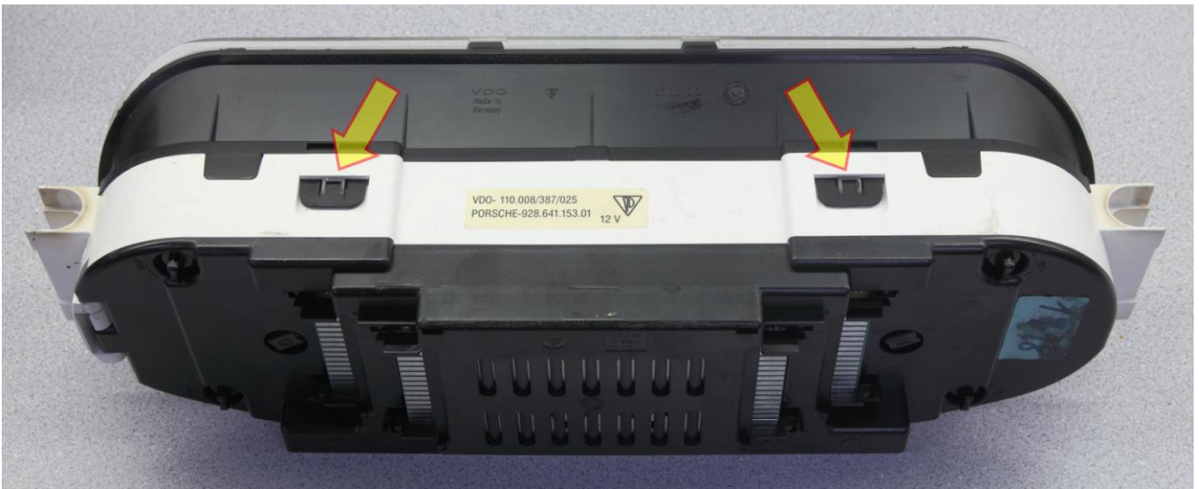
Figure 8: Two front-part-to-center-part-of-cluster latching fastening tabs on the bottom of the cluster
