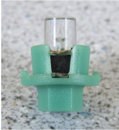
Figure 3: B8.4-XHP bulb; note base spread causing increased diameter near top of base
