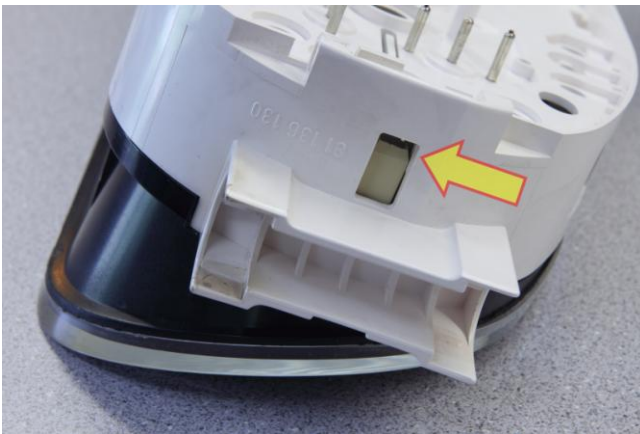
Figure 9: Slot to use for prying the front part from the center part of the cluster
