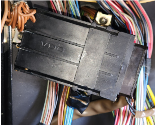
928.641.503.02 lamp controller located above fuse/relay panel
