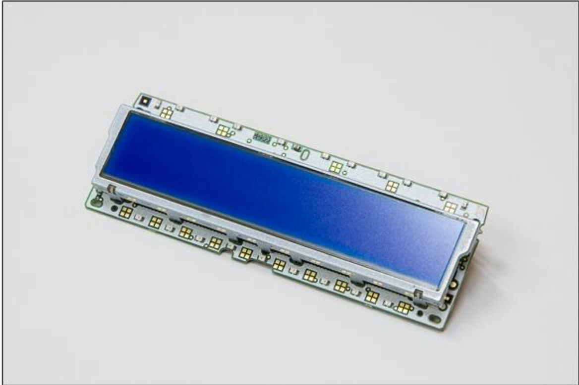
Front side of the Becker/BMW Radio Navigation Traffic Pro PCB with display:
