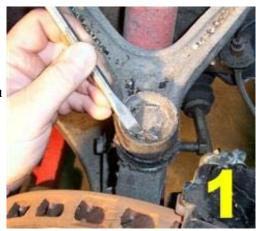
Step 3: The next step is to remove the nut that holds it to the spindle. You may find it is easier to get at the nut if you apply a little pre-load on the front suspension. In this picture, we've lifted the lower a-arm a little bit. It makes it easier to get behind the ball joint and at the nut to work on it. Also, turning the steering wheel hard left (or right) makes it easier too. You should find that a 19mm socket will fit nicely. Remove the nut.
