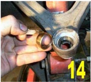
You may make a pushing tool with a wooden dowel if you like, but it is usually not necessary. The 928 Motorsports ball joint bushing is a precise fit into the Porsche 928 upper a-arm and you can press it in place with your fingers. It is all the way down when the top of the ball joint bushing is below the top of the inner lip inside the upper a-arm.
