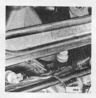
If the operating motor is not activated due to a fault, the rubber protective cap could be pulled off of the operating motor and the flaps opened manually with a knurled nut.
