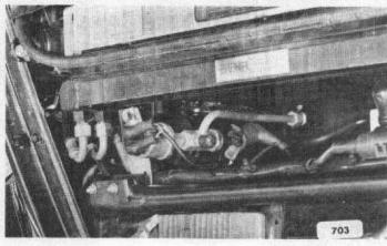
. . . and intake air temperature by way of temperature switch in intake manifold.
