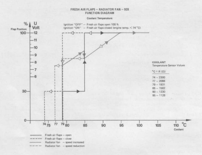
Flaps are always opened 100 % with the ignition turned off. If the ignition is turned on and the engine is cold (< 74 °C), the cooling air flaps will be closed.
