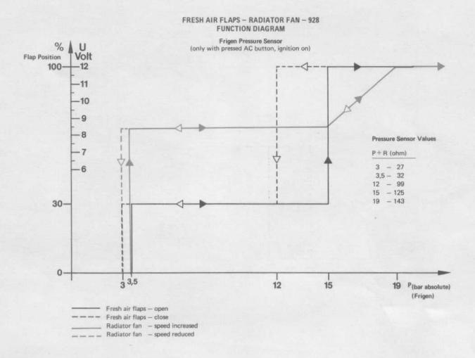
With the air conditioner switched on the cooling air flaps will be adjusted and the radiator fan motors switched on, depending on the refrigerant pressure in the high pressure line of the air conditioner, but independent of the coolant temperature.
