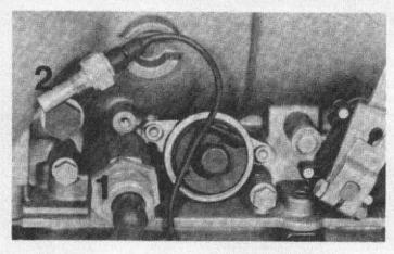
... refrigerant pressure of air conditioner by way of pressure sensor next to drier
